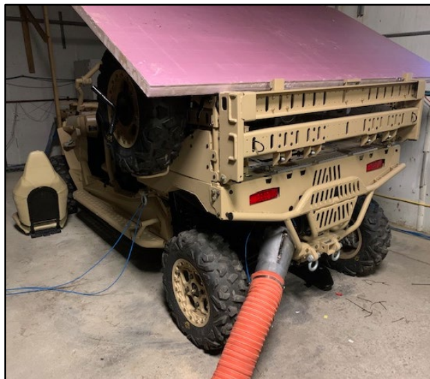
Figure 6. Exhaust hose connected to the tailpipe of the MRZR test vehicle.
